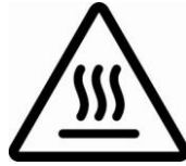
Temperature Hazard Caution or Warning
