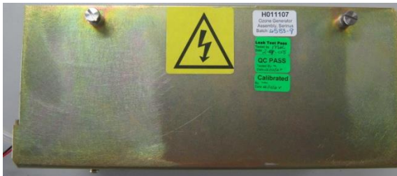
Figure 62 – Ozone generator assembly
