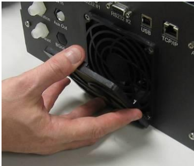
Figure 53 – Removing the fan filter
