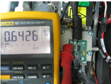
Figure 60 – Typical test point reading of cell pressure with vacuum connected to exhaust port
