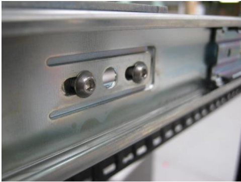
Figure 75 – Attach rack mount adaptors to outer slides
