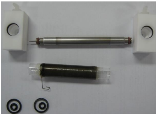
Figure 66 – Replacing Viton O-rings
