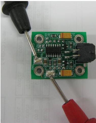
Figure 59 – Test point location
