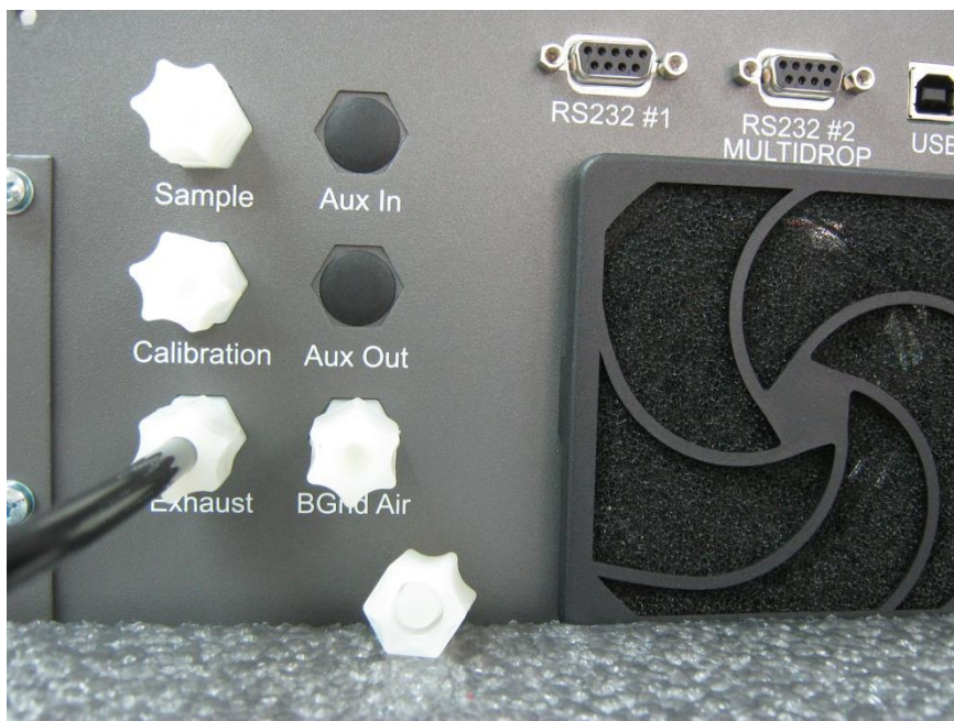
Figure 55 – Plugged Sample, Background, and Calibration Ports
