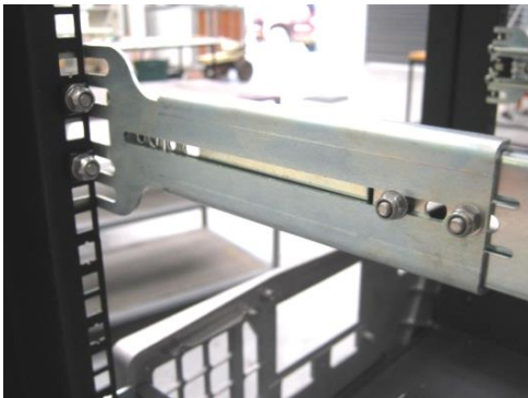
Figure 77 – Attach rack mount adaptors to outer slides
