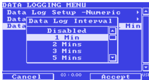
Figure 12 – Configure Serinus logging interval
