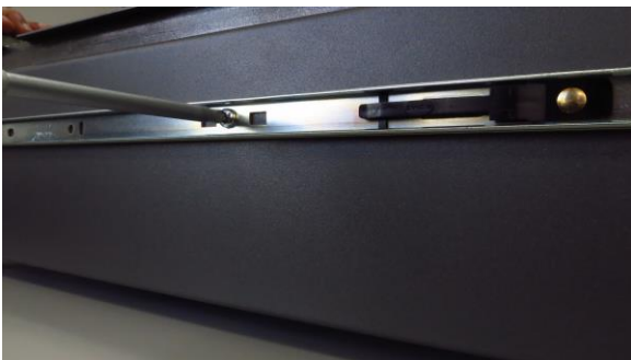
Figure 74 – Assemble inner slide on chassis
