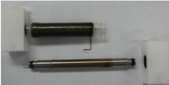
Figure 65 – Disassembled ozone generator cell assembly
