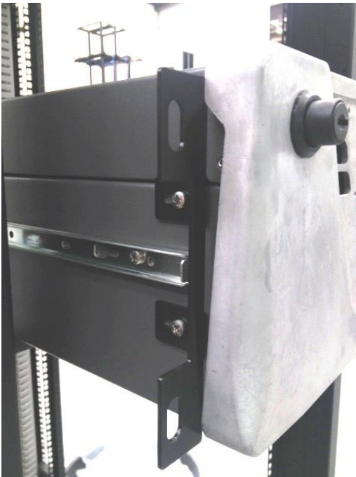
Figure 79 – Rack mount ears fitted to analyser
