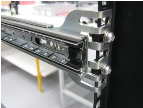
Figure 76 – Attach slides to front of rack
