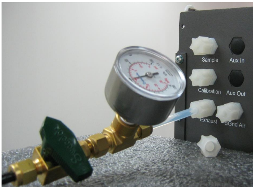
Figure 56 – Pressure gauge on exhaust
