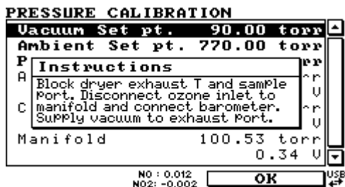
Figure 41 – Vacuum calibration, on-screen instructions
