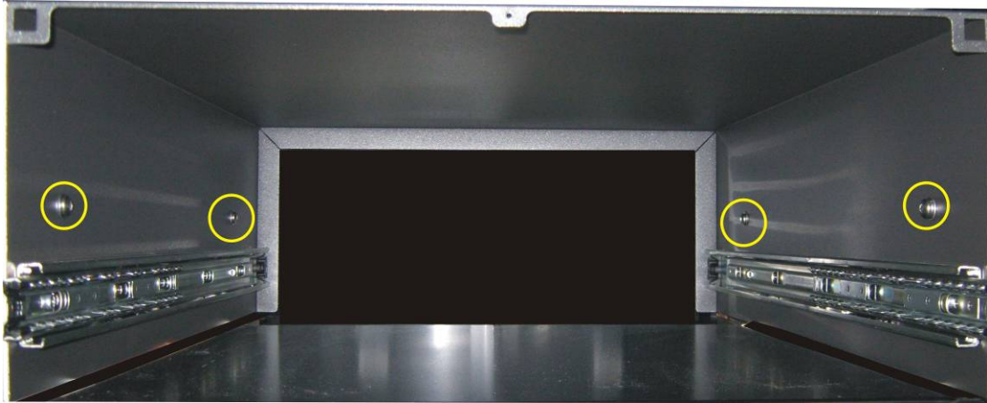
Figure 26 Installation of lid to rack mount brackets
