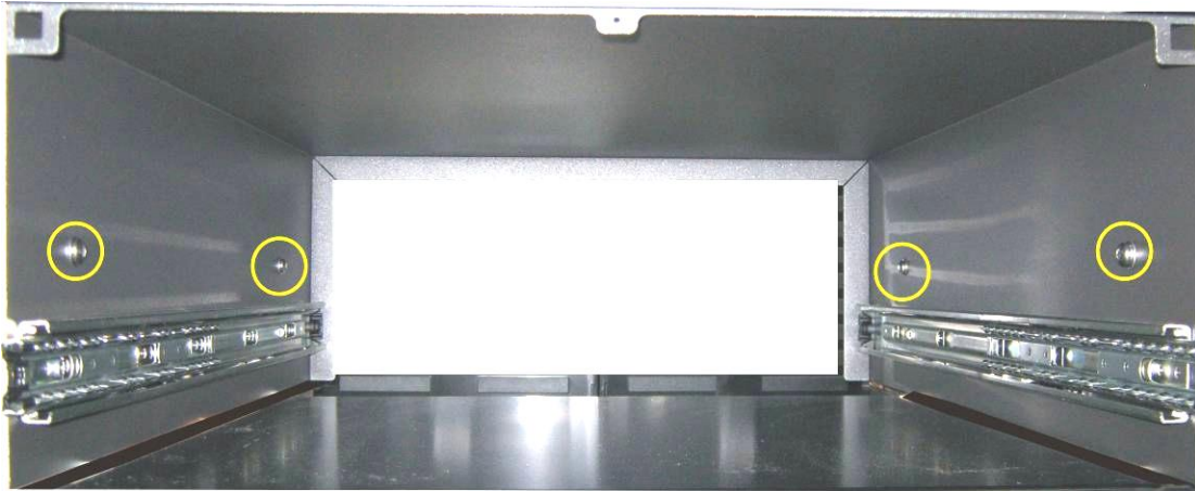
Figure 30 Installation of lid to rack mount brackets
