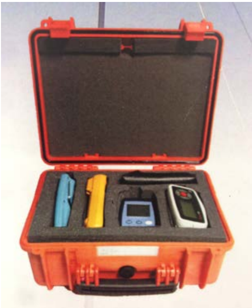
Figure 53 – Air Monitoring Test Equipment Kit (AMTEK) – Customisable
