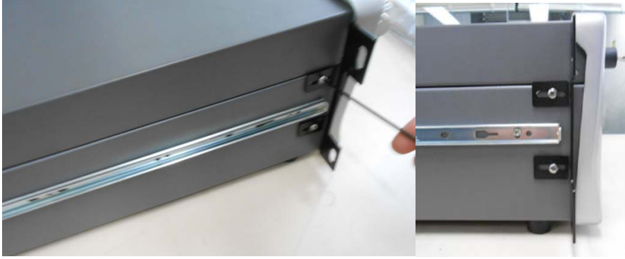
Figure 72 – Rack Mount Ears Fitted to Instrument
