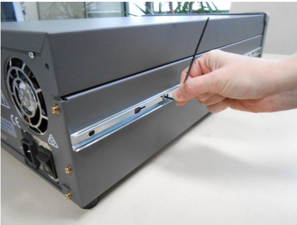
Figure 71 – Assemble Inner Slide on Chassis
