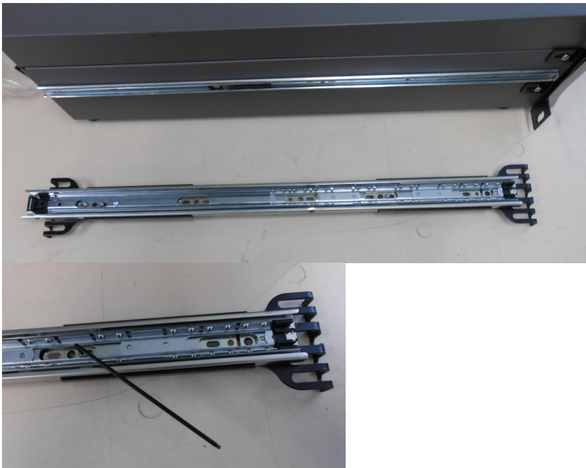
Figure 73 – Attach Rack Mount Adaptors to Outer Slides
