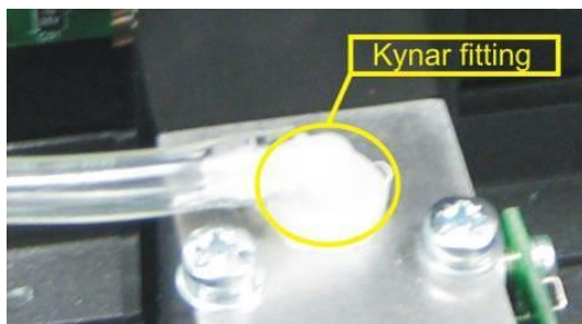
Figure 62 – Remove Kynar Fitting Containing Orifice
