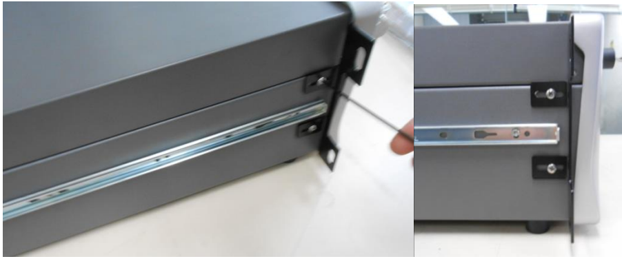
Figure 72 – Rack Mount Ears Fitted to Instrument
