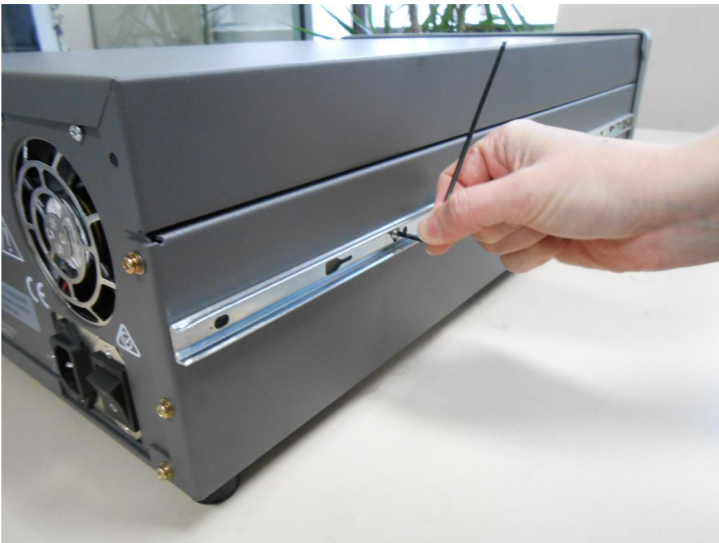
Figure 71 – Assemble Inner Slide on Chassis
