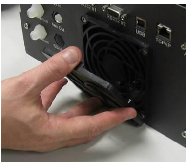
Figure 54 – Removing Fan Filter
