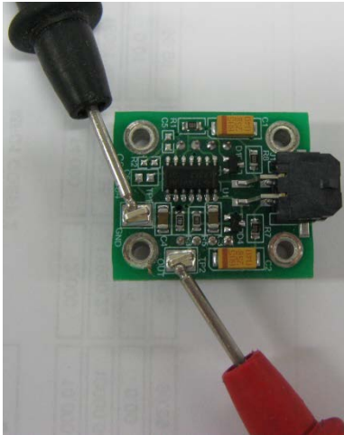
Figure 58 – Test Point Location
