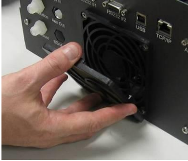
Figure 55 – Removing the Fan Filter
