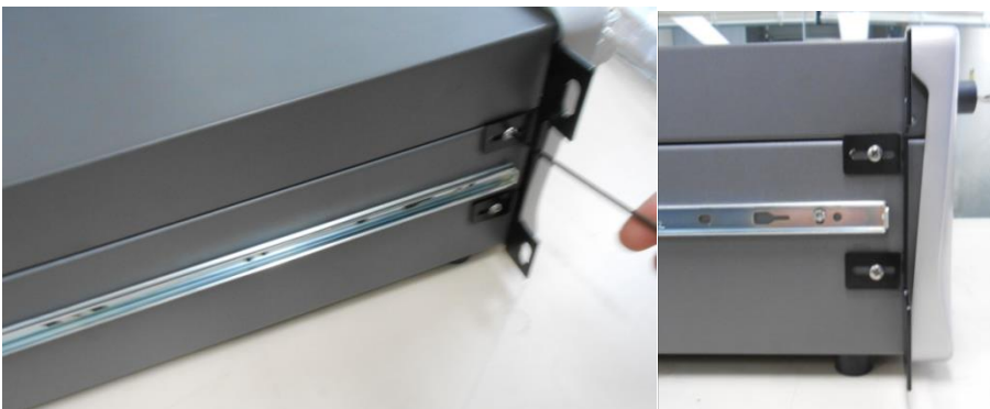
Figure 75 – Rack Mount Ears Fitted to Instrument
