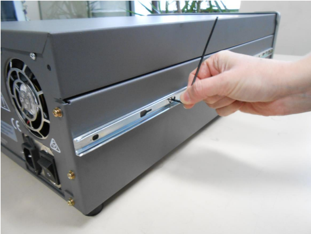
Figure 74 – Assemble Inner Slide on Chassis
