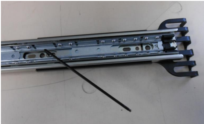
Figure 76 – Attach Rack Mount Adaptors to Outer Slides
