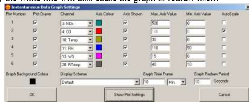
Figure 58 Instantaneous Graph Settings with Axis Settings
